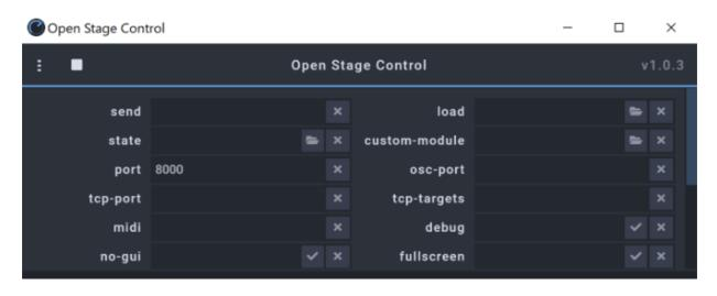
This needs to match the port that has been set in the corresponding OSCData line in the console. Port 8000 is the default. Afterwards the Open Stage Control session can be started.
